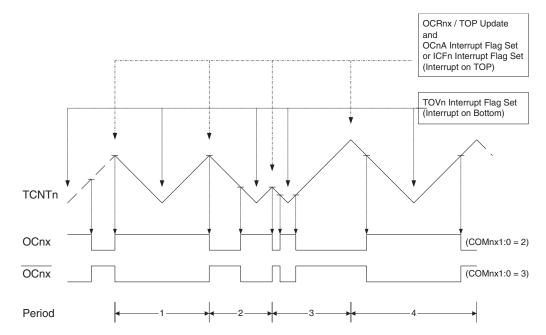
The Timer/Counter Overflow Flag (TOVn) is set each time the counter reaches BOTTOM. When either OCRnA or ICRn is used for defining the TOP value, the OCnA or ICFn flag is set accordingly at the same timer clock cycle as the OCRnx Registers are updated with the double buffer value (at TOP). The interrupt flags can be used to generate an interrupt each time the counter reaches the TOP or BOTTOM value.
