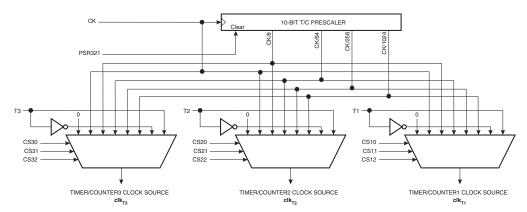
Figure 60. Prescaler for Timer/Counter1, Timer/Counter2, and Timer/Counter3
