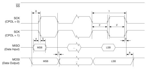
Figure 156. SPI Interface Timing Requirements (Slave Mode)
