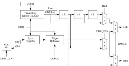
Figure 80. Clock Generation Logic, Block Diagram
