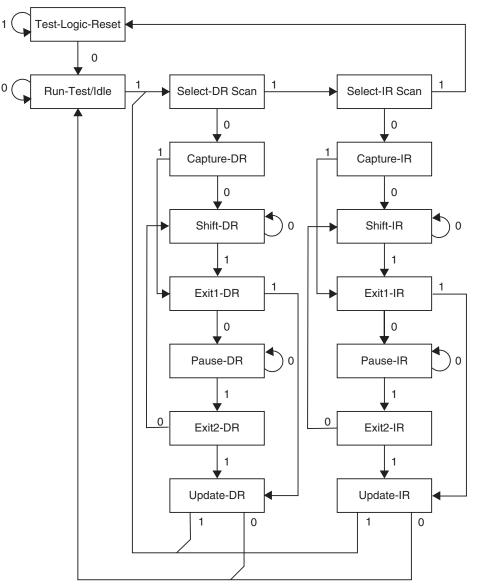
**TAP Controller**The TAP controller is a 16-state finite state machine that controls the operation of the Boundary-<br/>scan circuitry, JTAG programming circuitry, or On-chip Debug system. The state transitions<br/>depicted in Figure 121 depend on the signal present on TMS (shown adjacent to each state tran-<br/>sition) at the time of the rising edge at TCK. The initial state after a Power-on Reset is Test-<br/>Logic-Reset.
