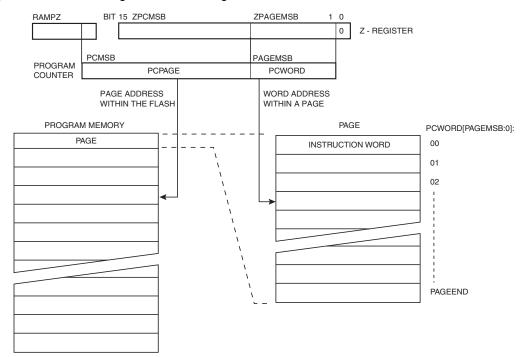
Figure 134. Addressing the Flash During SPM<sup>(1)</sup>
