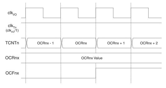
Figure 56 shows the same timing data, but with the prescaler enabled.
