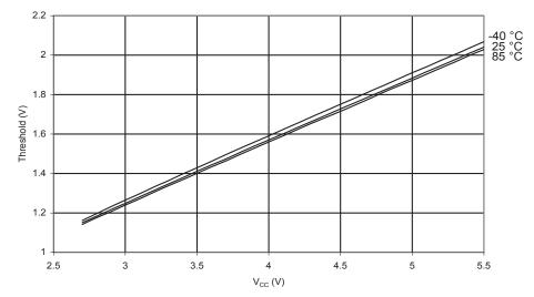
Figure 187. I/O Pin Input Threshold Voltage vs.  $V_{CC}$  (VIH, I/O Pin Read as '0')
