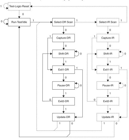
Figure 149. State Machine Sequence for Changing/Reading the Data Word
