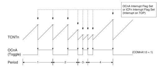
Figure 51. CTC Mode, Timing Diagram
