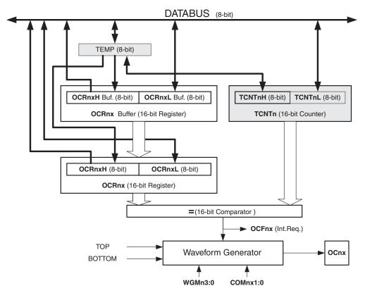
Figure 49. Output Compare Unit, Block Diagram
