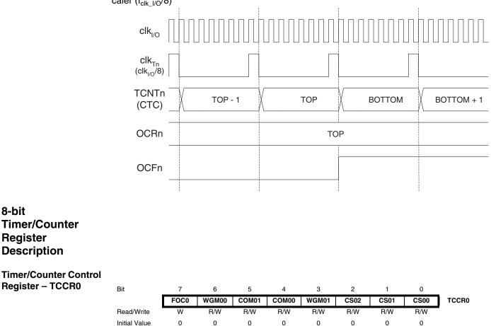
Figure 44. Timer/Counter Timing Diagram, Clear Timer on Compare Match Mode, with Prescaler (f<sub>clk I/O</sub>/8)
