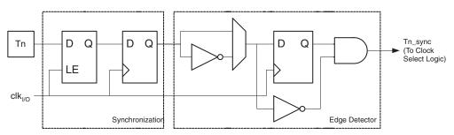
The synchronization and edge detector logic introduces a delay of 2.5 to 3.5 system clock cycles from an edge has been applied to the Tn pin to the counter is updated.
