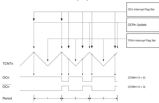
Figure 40. Phase Correct PWM Mode, Timing Diagram
