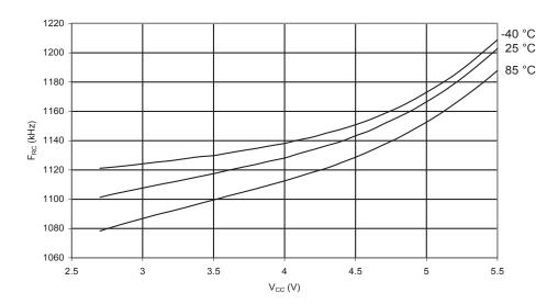
Figure 193. Calibrated 1MHz RC Oscillator Frequency vs. Temperature
