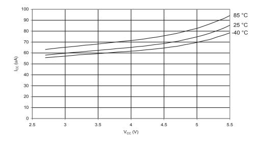
Figure 209. Programming Current vs.  $V_{CC}$
