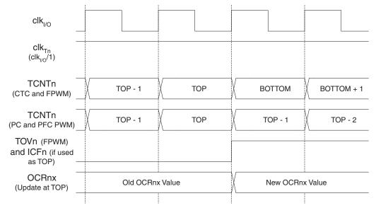
Figure 57. Timer/Counter Timing Diagram, no Prescaling
