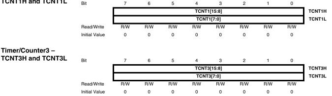
The two *Timer/Counter* I/O locations (TCNTnH and TCNTnL, combined TCNTn) give direct access, both for read and for write operations, to the Timer/Counter unit 16-bit counter. To ensure that both the high and low bytes are read and written simultaneously when the CPU accesses these registers, the access is performed using an 8-bit temporary High Byte Register (TEMP). This Temporary Register is shared by all the other 16-bit registers. See "Accessing 16-bit Registers" on page 114.
