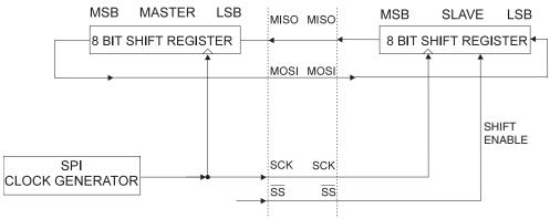
Figure 76. SPI Master-Slave Interconnection
