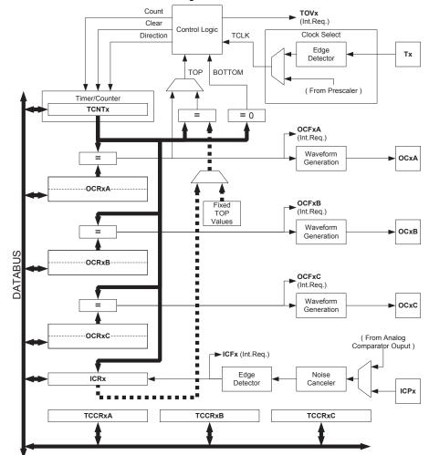
Figure 46. 16-bit Timer/Counter Block Diagram
