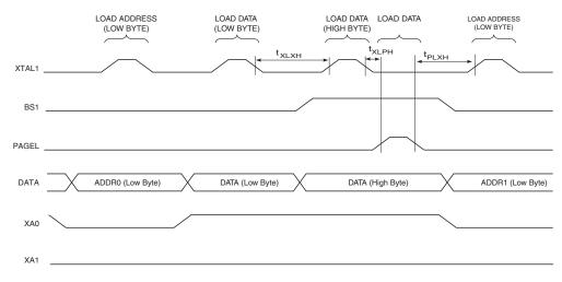
Figure 142. Parallel Programming Timing, Loading Sequence with Timing Requirements
