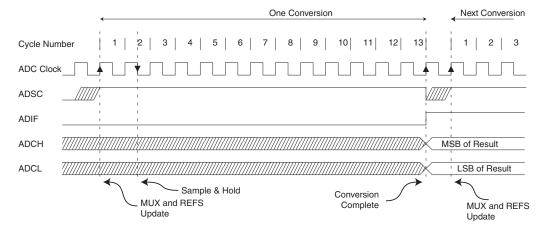
Figure 112. ADC Timing Diagram, Free Running Conversion
