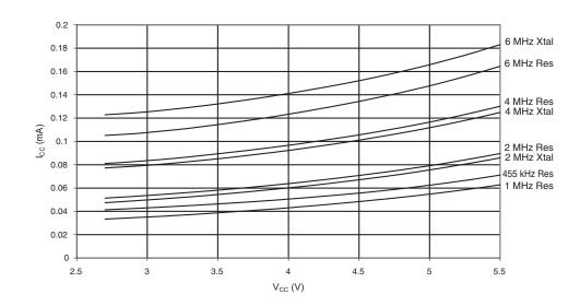
Figure 179. Standby Supply Current vs. V<sub>CC</sub> (CKOPT programmed)
