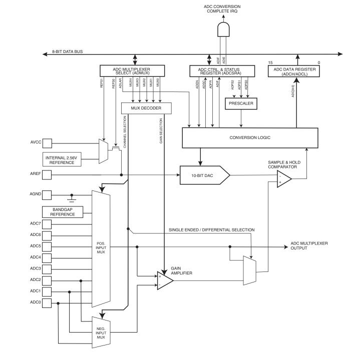
Figure 108. Analog to Digital Converter Block Schematic
