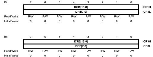
The Input Capture is updated with the counter (TCNTn) value each time an event occurs on the ICPn pin (or optionally on the Analog Comparator Output for Timer/Counter1). The Input Capture can be used for defining the counter TOP value.
