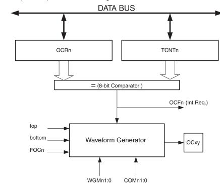
Figure 36. Output Compare Unit, Block Diagram
