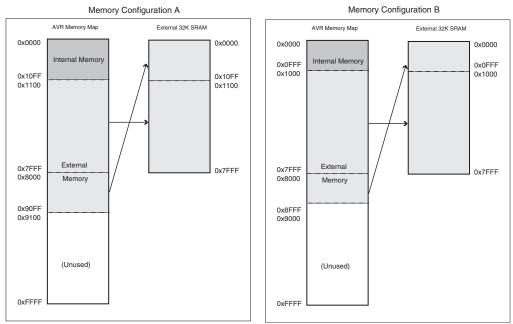
Figure 17. Address Map with 32 Kbyte External Memory
