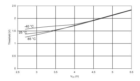
Figure 214. Reset Input Threshold Voltage vs. V<sub>CC</sub> (VIH, Reset Pin Read as '1')
