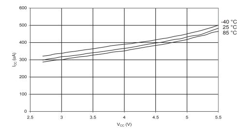
Figure 207. ADC Current vs.  $AV_{CC}$  (ADC at 1MHz)
