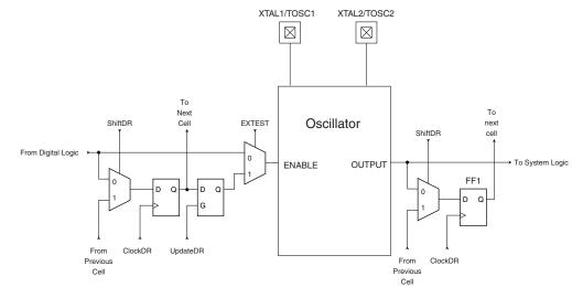
Figure 128. Boundary-scan Cells for Oscillators and Clock Options
