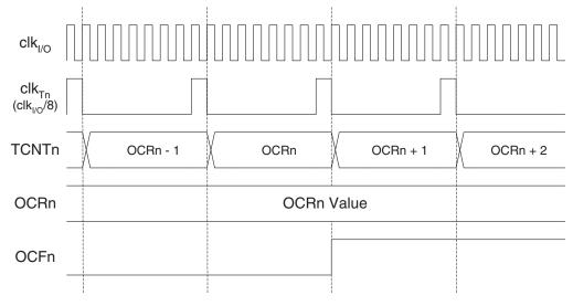
Figure 44 shows the setting of OCF0 and the clearing of TCNT0 in CTC mode.
