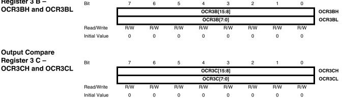
The Output Compare Registers contain a 16-bit value that is continuously compared with the counter value (TCNTn). A match can be used to generate an output compare interrupt, or to generate a waveform output on the OCnx pin.
