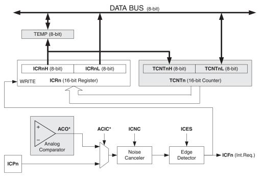
Figure 48. Input Capture Unit Block Diagram
