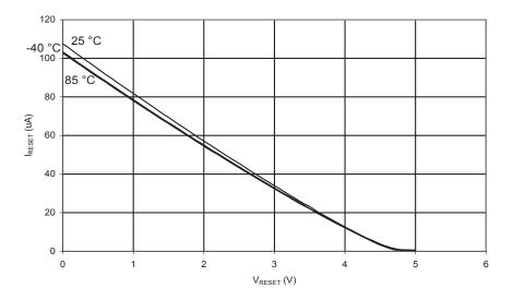
Figure 213. Reset Pull-up Resistor Current vs. Reset Pin Voltage ( $V_{CC}$  = 2.7V
