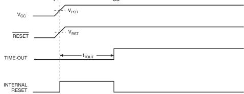
Figure 23. MCU Start-up, RESET Tied to V<sub>CC</sub>.
