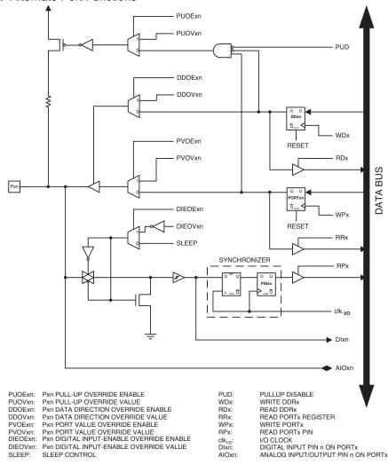
Figure 33. Alternate Port Functions<sup>(1)</sup>
