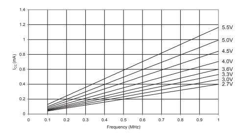
Figure 169. Idle Supply Current vs. Frequency (1 - 20MHz)
